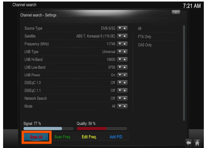
[Picture 4] Select "DCVB-S/S2, ATSC" or "Source Type" which is fit with region. and adjust "Satellite" as you want and click "Scan All".
